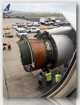
warnings of an engine compressor stall, and shut down the engine. The crew declared an emergency and proceeded to KHNL without further incident.
