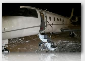
activated, causing the door to blow open violently when unlatched. There were no other injuries. Aircraft damage was limited to the door and its frame and described as "minor."
